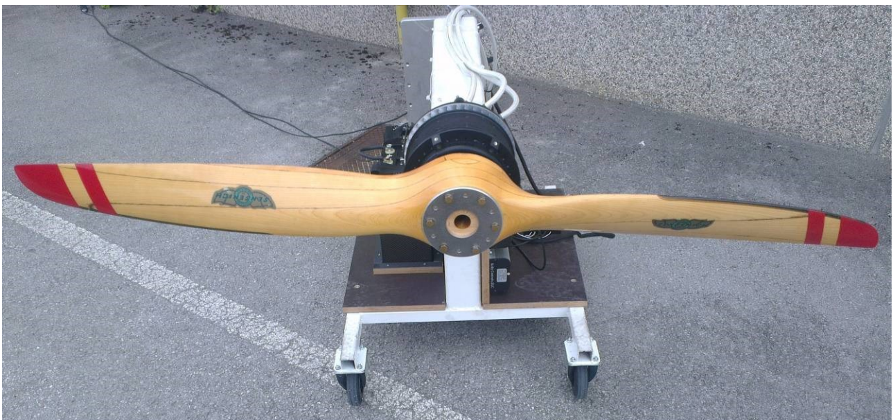
FES M130 motor mounted on test bench with a wooden propeller
