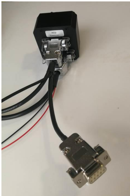
DB9 female connector to FCU
