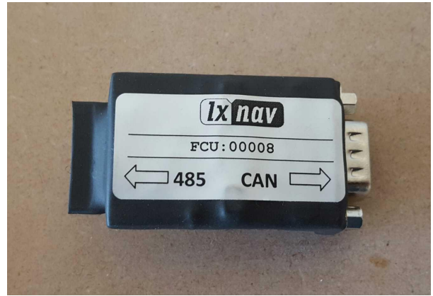
FES Bridge, back view
